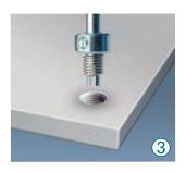
Now in the third step, the recoil wire thread insert will be screwed with the screwing tool.
