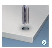
In step two in the new hole will be cutting a thread with the thread tap.
